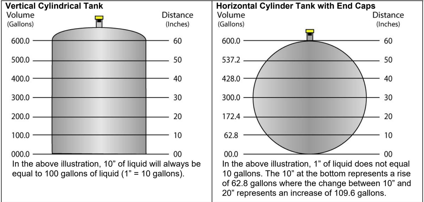
When volume is selected, the 4-20 mA output from the sensor will be proportional to the volume of the tank, not the height of the tank. This means that the current output will track the volume of the tank (in gallons or liters) within a non-linear tank (Vertical Cylinder Tank with Cone Bottom, Horizontal Cylinder Tank with End Caps, Horizontal Cylinder Tank with Spherical End Caps or Spherical Tank).
