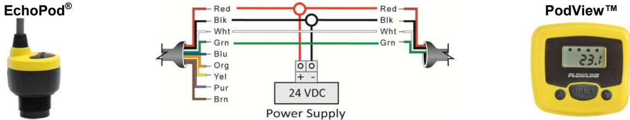
**Wiring is identical for all EchoPod® models – Use only the Red, Black, Green and White wires.**
