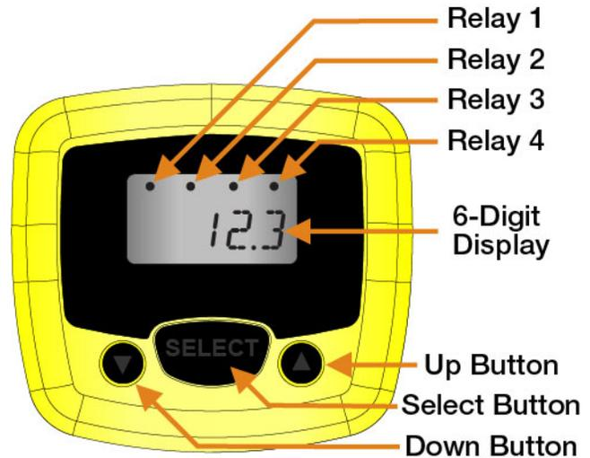
**Note:** To increase the scrolling speed of the display, hold down the SELECT button while simultaneously pressing the UP or DOWN button.
