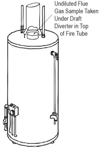
Domestic hot water tanks with the 'bell' shaped draft diverter can be accurately tested by inserting the probe tip directly into the top of the fire tube below the diverter.
