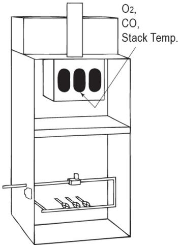
For atmospheric burner or gravity vented, forced air heating equipment with a clamshell or sectional heat exchanger design, test each of the exhaust ports at the top of the heat exchanger. The probe should be inserted back into each of the exhaust ports to obtain a flue gas sample, before any dilution air is mixed in.
