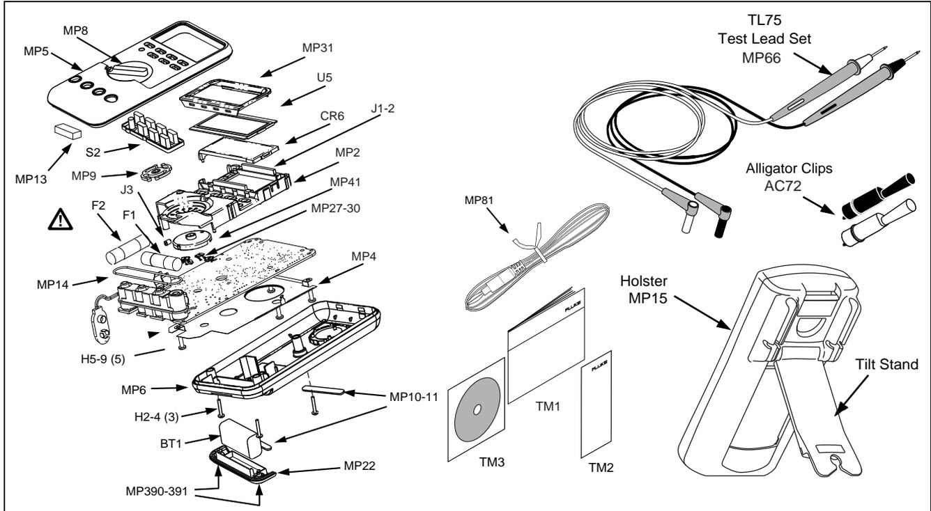
Figure 12. Replaceable Parts
