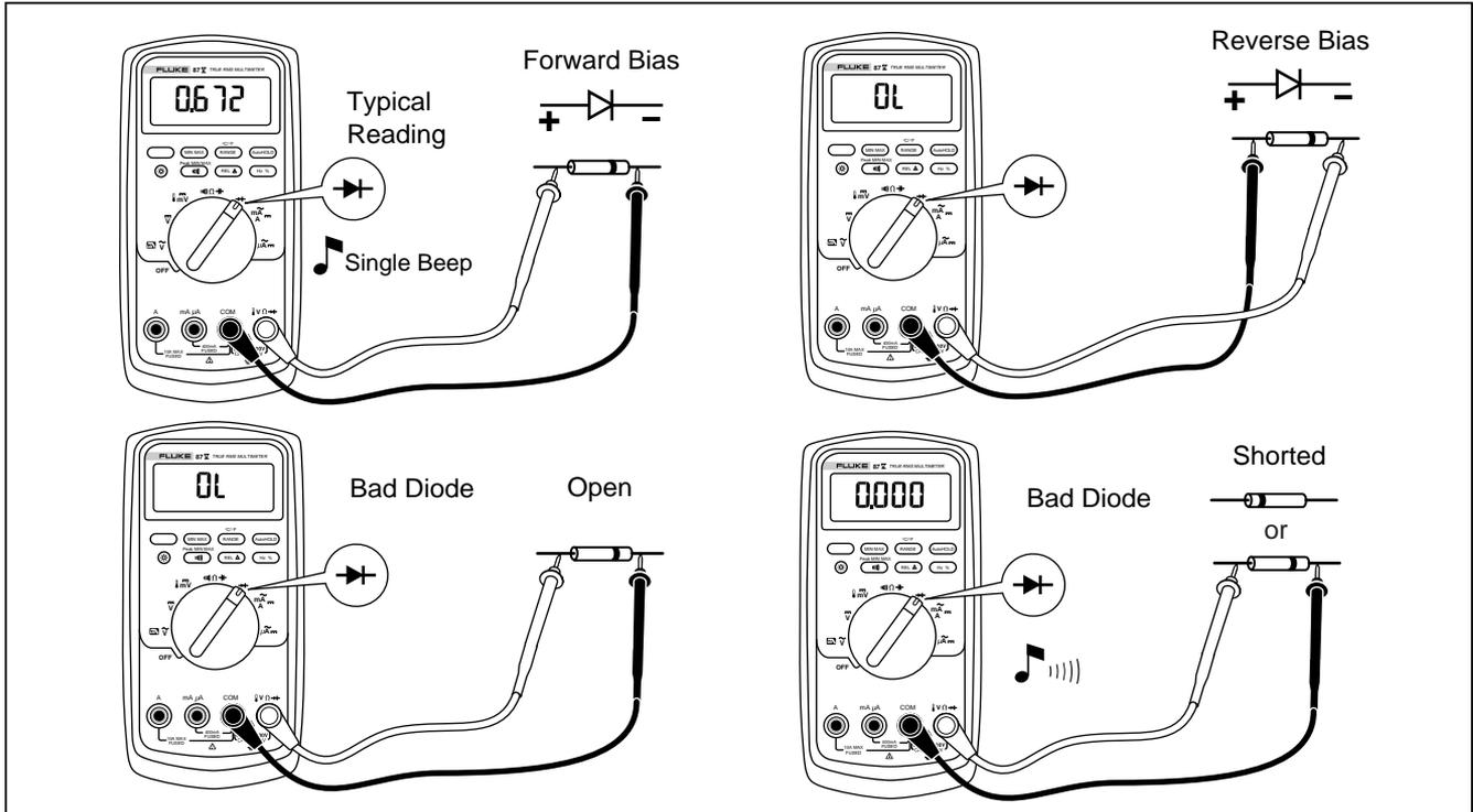
Figure 7. Testing a Diode
