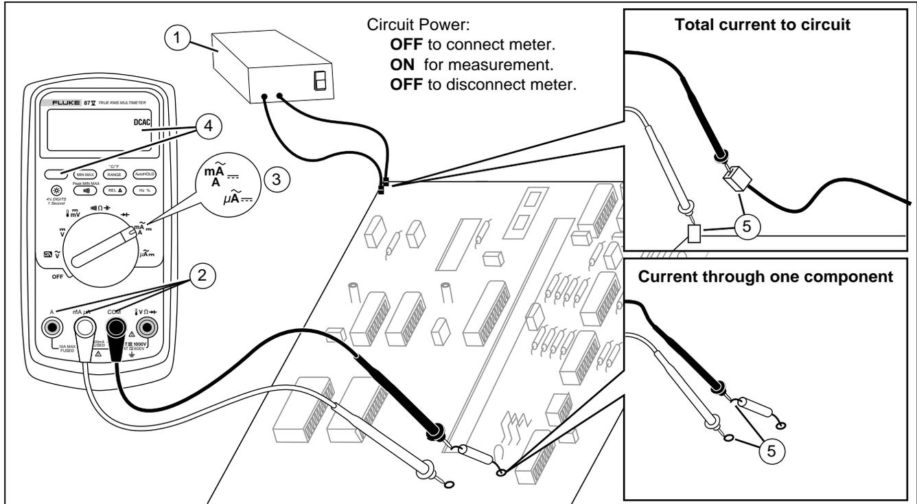
Figure 8. Measuring Current
