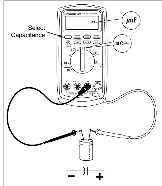
Figure 6. Measuring Capacitance
