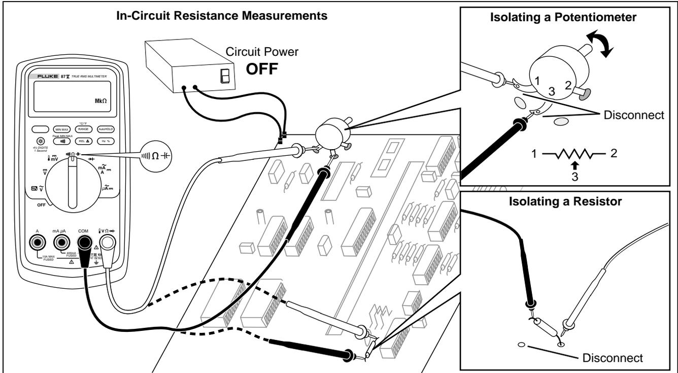
Figure 5. Measuring Resistance
