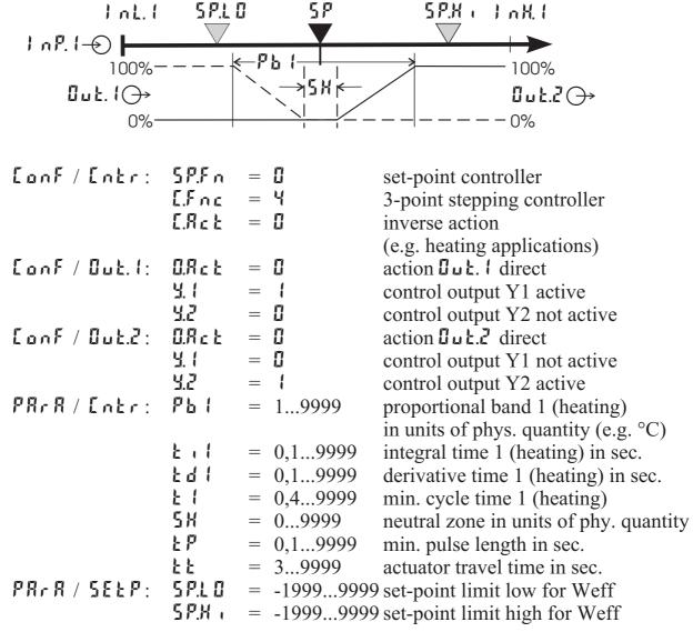
For direct action of the 3-point stepping controller, the controller output action must be changed ( Lanf / Lnkr / Lnkr = 1).
