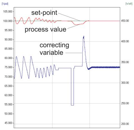
With a *3-point controller*, optimization for the "heating" or "cooling" parameters occurs dependent of the instantaneous condition.
