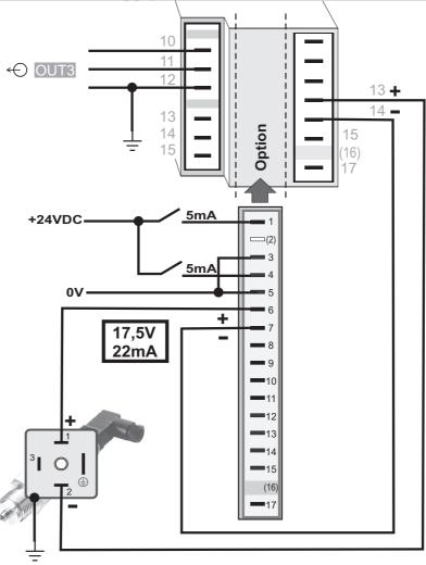
Analog outputs OUT3 or OUT4 and transmitter supply  $U_T$  are connected to different voltage potentials. Therefore, take care not to make an external galvanic connection between OUT3/4 and U<sub>T</sub> with analog outputs!
