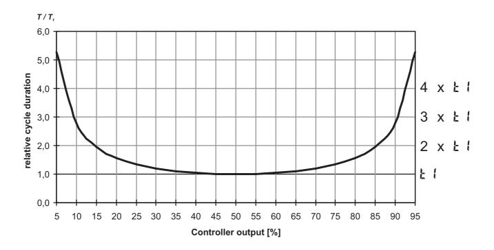
Parameters to be adjusted: L: min. cycle time 1 (heating) [s] (PRr R/LnEr) L: min. cycle time 2 (cooling) [s]
