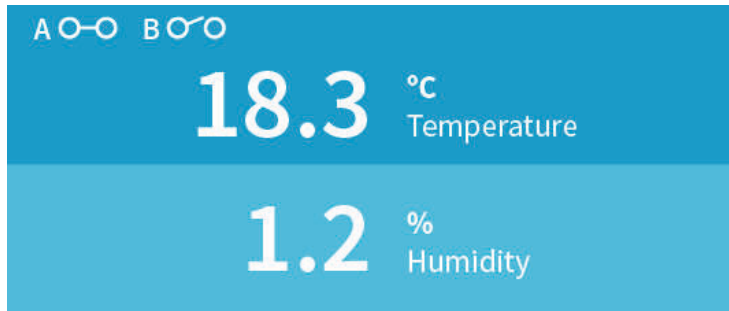
Figure 21 Relay Icons on the Optional Display (Relay A Active, Relay B Not Active)
