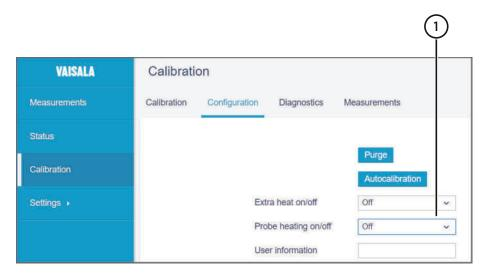
Figure 27 Probe Heating Options in Configuration Tab
