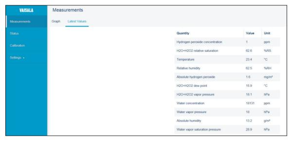
Figure 18 Latest Values Tab, H<sub>2</sub>O<sub>2</sub> Probe Example (Desktop Browser)
