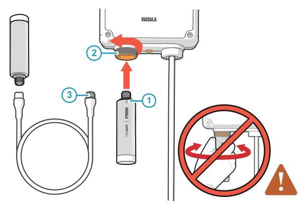
Figure 11 Attaching Probes and Cables to Indigo
