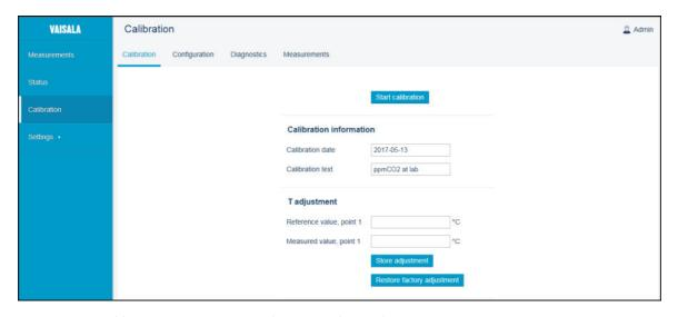
Figure 20 Calibration Menu (CO<sub>2</sub> Probe Example, Desktop Browser)
