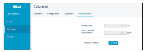
Figure 30 Measurements Tab, CO<sub>2</sub> Probe Example
