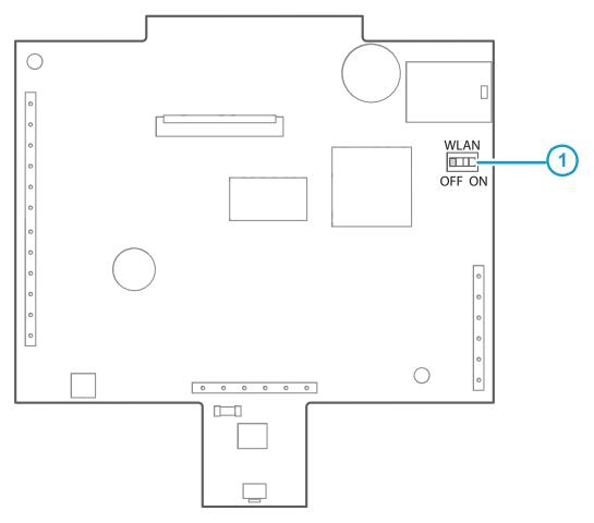
Figure 12 WLAN OFF/ON DIP Switch on Indigo Circuit Board
