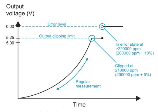
Figure 22 Example of Analog Output Overrange Behavior
