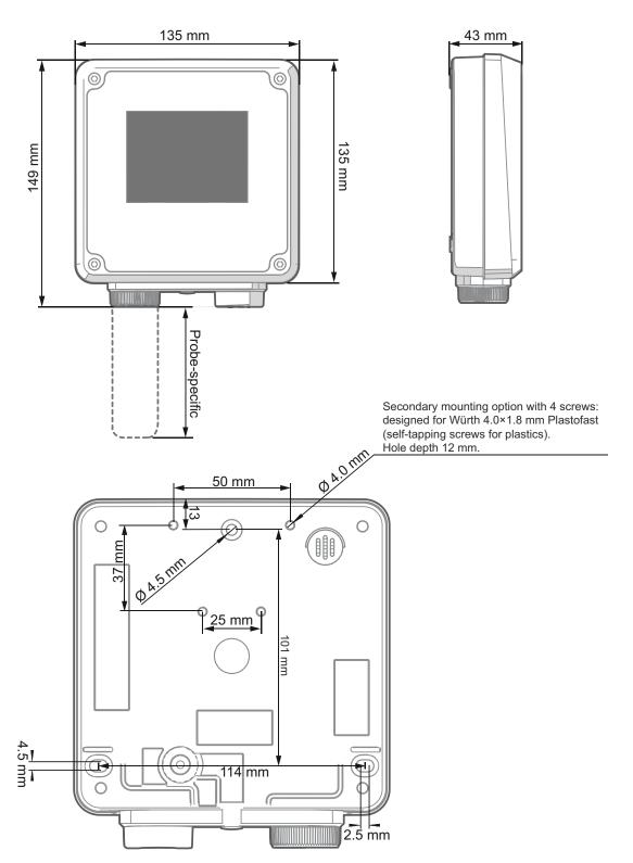
Figure 34 Indigo Transmitter Dimensions in Millimeters (mm)
