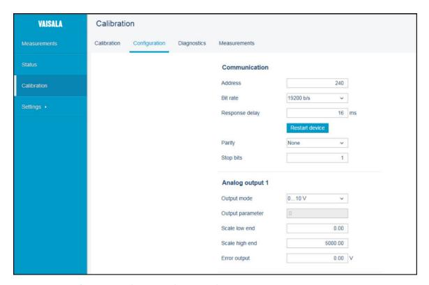
Figure 32 Configuration Tab, CO<sub>2</sub> Probe Example
