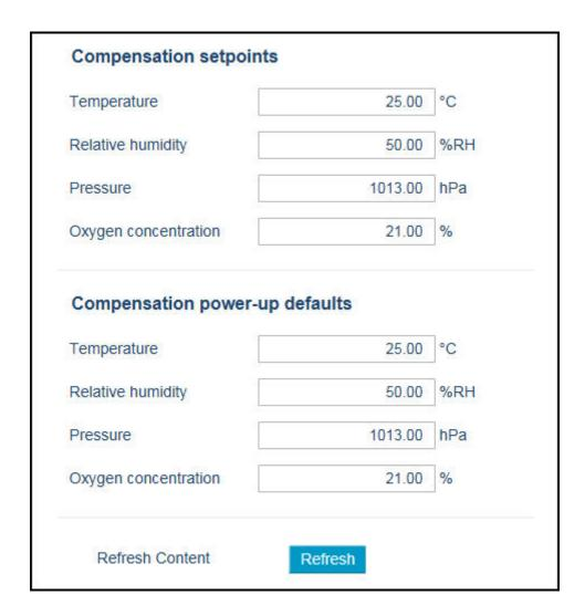
Figure 29 Compensation Setpoint and Power-Up Default Selection, CO<sub>2</sub> Probe Example
