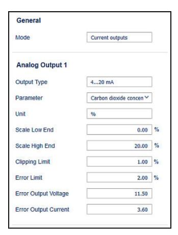
Figure 21 Analog Output Configuration Options
