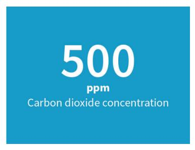
Figure 3 Indigo 201 Display with One Parameter
