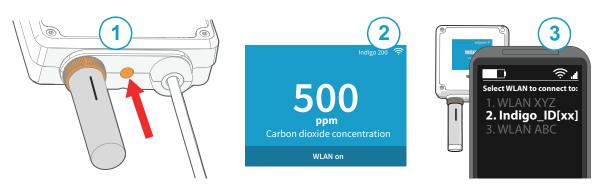
Figure 14 Enabling and Accessing Indigo's Wireless Configuration Interface
