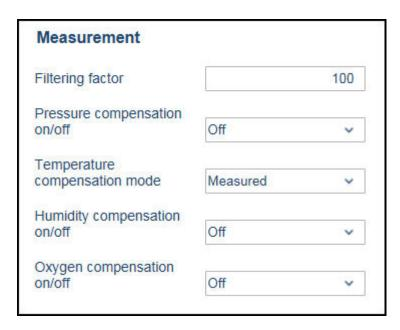
Figure 28 Measurement Selections, CO<sub>2</sub> Probe Example
