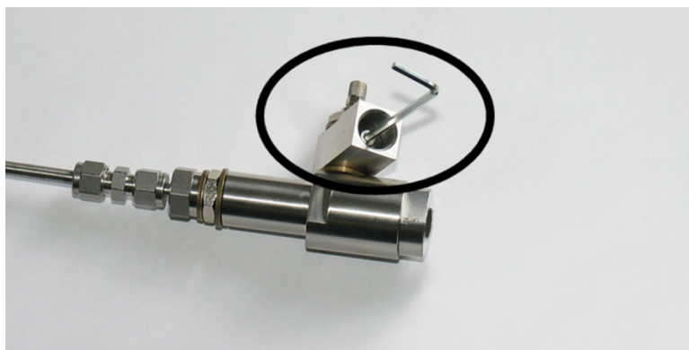
Figure 17 Removing the Leak Screw
