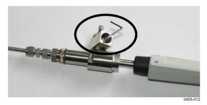
Figure 30 Removing the Leak Screw
