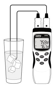
The DTK2 has an automatic ice-point calibration function. Please follow these steps to calibrate your meter to the thermocouple probes.
