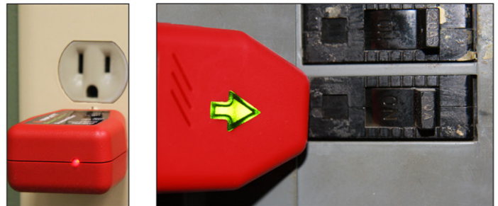
Identify breaker locations with bright LED visual and audible indication
