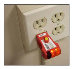
To test, simply plug into receptacle and observe the light pattern — Fault charts are located on both sides of the tester so that it can easily be used on receptacles in "ground up" or "ground down" installations
