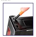
To open meter, insert a flat head screwdriver or similar instrument in both slots on the side of the cover and pry open. The UM-Series meters slide out from the front of the case as a complete assembly.
