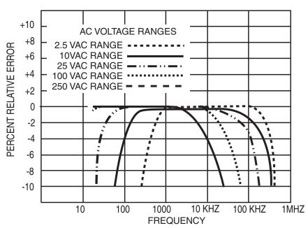
Figure 4-1. Typical Frequency Response, AC Voltage Ranges
