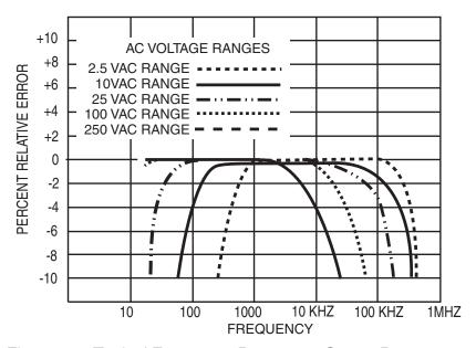
Figure 4-2. Typical Frequency Response, Output Ranges
