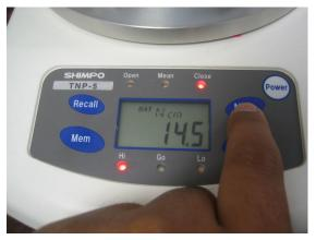
Picture above indicates the memory ID followed by the stored data. Pressing the mode button anytime exits out of the memory window. Below is a flowchart of how the recall function works.
