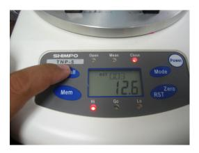
Example from the picture above shows 3 data is saved (003) and the last value is 12.6. Pressing the Zero/RST button, the last data is eliminated (CLr will appear on the screen). Pressing the Zero/RST button again deletes the next data stored in the TNP torque meter.
