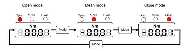
Pressing the Mode key toggles through the mode available from the TNP, LED indicators are provided to display current selected mode.
