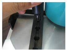
It is important to make sure that all the jigs are flush to the moving brackets. Each one of these jigs has set pins which slides into place inside the grooved brackets.
