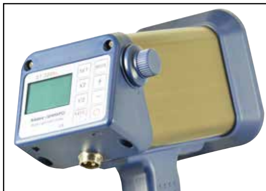
Operation Panel & Flash Adjustment Dial
