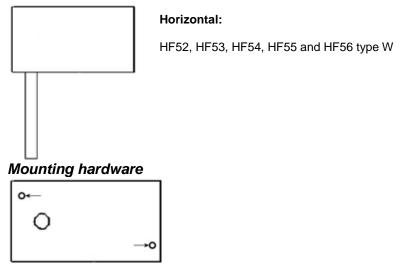
**Method 1**: The HF5 is supplied with 2 screws, 2 drywall anchors and two rubber washers. The base of the enclosure has 2 screw-wells (see drawing) that are normally closed at the bottom. Use the template provided with the HF5 to drill mounting holes in the wall and insert the drywall anchors. Place a rubber washer on each screw. Insert a screw in each well and push to open the bottom of the well.
