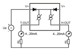
The maximum permissible cable length connecting the HF52 to other devices is determined by the total resistance resulting from the addition of the cable resistance and that of the devices connected in series with the unit.
