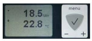
Except for the HF52 (2-wire circuit type), the LC display of the HF5 has a backlight.
