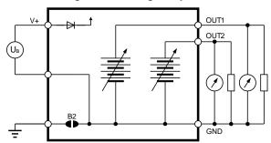
The maximum permissible cable length can be determined under consideration of the voltage drop caused by the current flowing to the devices connected to the unit. The voltage drop in the cable depends both on cable resistance and on the equivalent resistance of the devices connected in parallel to the unit. The total resistance connected to each unit output should be at least 1000  $\Omega$ . Cable resistance should not be more than 1/1000 of the load resistance.
