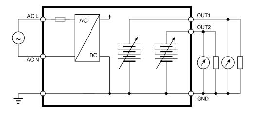
The maximum permissible cable length can be determined under consideration of the voltage drop on the cable.
