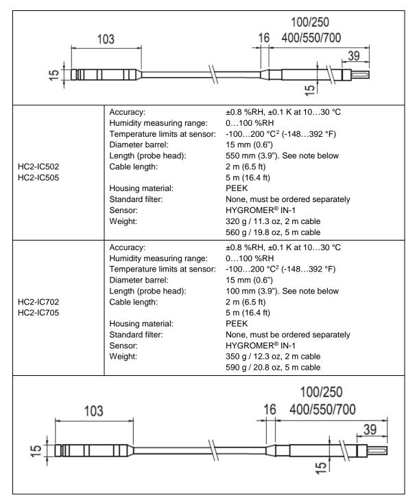
$<sup>^2</sup>$  Rotronic probes allow a peak load of 3x5 minutes at 200  $^{\circ}$ C without suffering any permanent damage. The time between the peak
