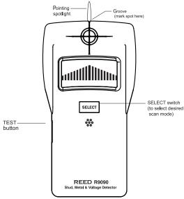
Press TEST button for about 2 seconds to turn on the unit.
