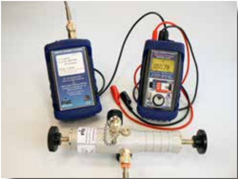
PIE 830 with Pressure Module, Pressure/Vacuum Pump & Hose
