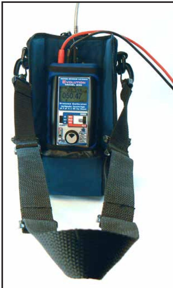
Hands free carrying case with pockets for the PIE 830 and the Pressure Module. Back of case has zippered pocket for the manual, test leads, hoses & pressure fittings.
