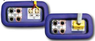
Simulating or reading RTDs uses copper wire.
