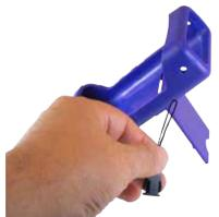
Remove the PIE Calibrator from the boot and disconnect the two loops from the ends of the strap.
