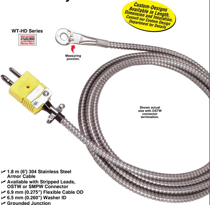
Rugged thermocouple, for surface mount applications, has a washer mounting surface and an overall dimension of 17.3 mm (0.680") OD, with a 6.6 mm (0.260") mounting hole of 304 SS material. Attached to the mounting surface: 1.8 m (6') of 304 SS flexible armor cable with stripped wire ends. Armor cable has 6.9 mm (0.275") OD, with 1.78 mm (0.070") washer thickness. Standard male connectors are available for cold-end termination. Rated to 480°C (900°F) for Type K only.
