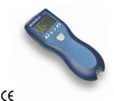
The *Pocket Tach 99 (PT99)* is a digital, battery-powered portable non-contact optical tachometer, which operates up to 36 inches from a reflective target using a bright red LED light source. The ergonomic design allows safe, direct line-of-sight viewing of both the rotating target and the display at the same time, while providing a non-slip rubber surface for single hand operation. The **PT99** is the value-leader of the world-class Pocket Tach Series from Monarch.
