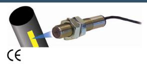
*IRS (Infrared Sensor):* Ideal sensor for working up to 0.5" (12mm) from high speed equipment or other applications providing only contrasting light and dark surfaces or beam interruption by solid objects as small as 0.30" (1mm).
