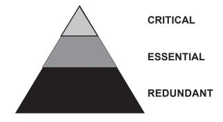
**Critical Machines** expensive premium equipment, generally >500 HP. Usually less than 5% of all plant equipment. Maintenance dollars per horsepower per year average \$11.00. This category of equipment is very well maintained and monitored. Continuous monitoring systems are better suited for this type of equipment.
