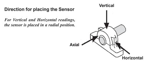
Also establish a starting point for each machine. Begin from the OUTBOARD END of the DRIVE UNIT, calling this point A. Proceed to label Points (bearings) as needed until you have reached the outboard end of the driven unit.
