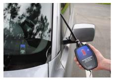
Place the Tone Generator inside vehicle, closed vessel, container or building to locate leaking seals and gaskets.
