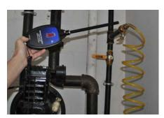
Locate pin-hole leaks up to 10 feet away. Find pressurized or vacuum leaks on all types of gases such as air, Freon, nitrogen, propane, etc.
