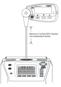
For best results, allow ample time for the probe to stabilize before recording measurements. The stability display is helpful for this.
