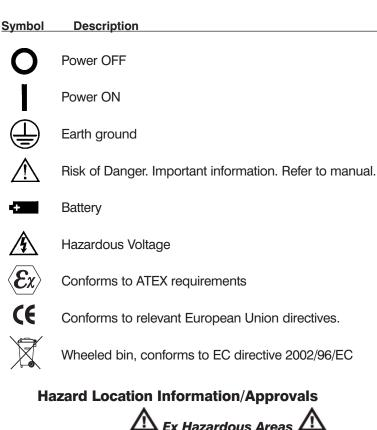
An Ex-hazardous area as used in this manual refers to an area made hazardous by the potential presence of flammable or explosive vapors.
