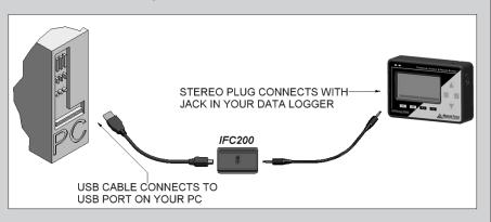
Insert the USB connector of the IFC200 into an available USB port. Fully insert male connector of the IFC200 interface cable into the female receptacle of the data logger\*.
