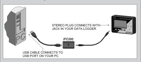
Fully insert the male connector of the IFC200 interface cable into the female receptacle of the data logger. Fully insert the female USB connector into the USB.
