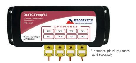
The OctTCTempV2 is an 8-channel thermocouple data logger with a reading rate of up to 4 Hz. It can measure and record 130,944 readings per channel. To maximize memory capacity, users can enable or disable channels. For easy identification, each channel can be named with up to a ten digit title.
