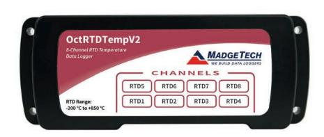
The OctRTDTempV2 is an 8-channel, RTD based temperature data logger with a reading rate of up to 4 Hz. It can measure and record up to 174,592 readings per channel. To maximize memory capacity, users can enable or disable channels. For easy identification, each channel can be named with up to a ten digit title. The storage medium is non-volatile solid state memory, providing maximum data security even if the battery becomes discharged. The OctRTDTempV2 makes data retrieval quick and easy.
