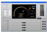
The design software provides a number of building blocks which allow users to drag-and-drop elements onto the screen to quickly create advanced user interfaces. From background images to text elements, analogue style meters, touch-screen navigation elements through to maths and logic functions, data logging and serial communications, users can build up multi-screen interfaces without needing to write a line of code.
