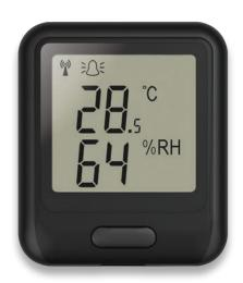
During configuration, the sensor will search for an existing wireless network whilst physically connected to the PC. It can then be placed anywhere within range of the network. If the sensor temporarily loses connectivity with the network, it will log readings until it is able to communicate again with the PC application or FilesThruTheAir™ Cloud (max 30 days at 10 second sample interval).
