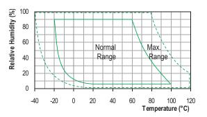
Long term exposure to humidity levels outside of the 'normal' range may temporarily offset RH measurements (±3%RH after 60 hours). Once returned to less extreme conditions the device will slowly return towards calibration state.
