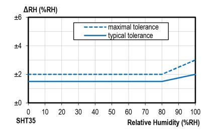
Typical tolerance of RH over Temperature:
