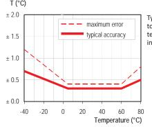
Typical and maximal tolerance for temperature sensor
