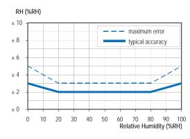
Typical and maximal tolerance at 25°C for relative humidity.
