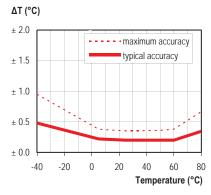
Typical and maximal tolerance for temperature sensor
