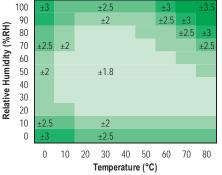
Typical accuracy of relative humidity measurements given in %RH for temperatures 0 to
