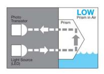
When the liquid level falls below the prism, light from the infrared LED is reflected back into the prism and onto the photo transistor. The electronic switch then opens the circuit.
