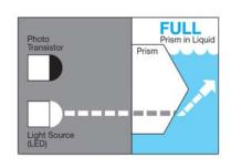
When the prism is immersed in liquid, light from the infrared LED is refracted into the liquid and fails to activate the internal photo transistor. The electronic switch then closes the circuit.
