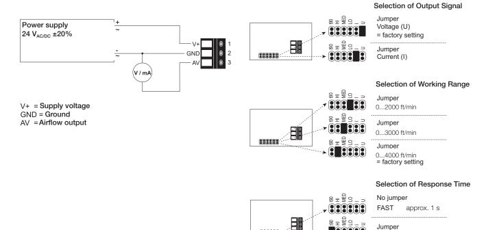
The output signal, working range and response time are selected via the jumpers according to the picture.
