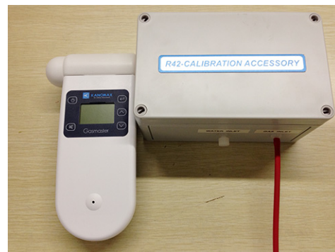
Use this orientation for calibrating CO
