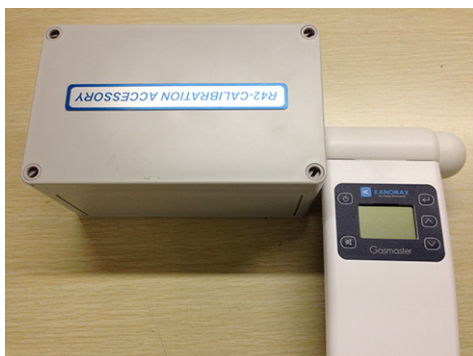
Use this orientation for calibrating PID and CO 2
