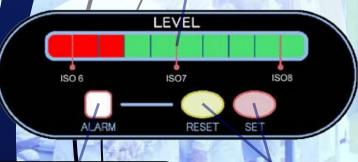
Alarm comes on when the setting level goes beyond the required cleanliness level while monitor gives alarm signal ouput.
