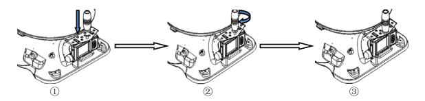
Note: The support poles and the portable handle should be disassembled before packing the capture hood in the carrying case to avoid damaging the case.
