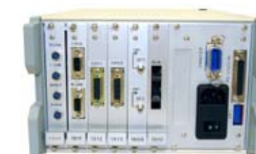
Model 1560 has 6 slots for modules
