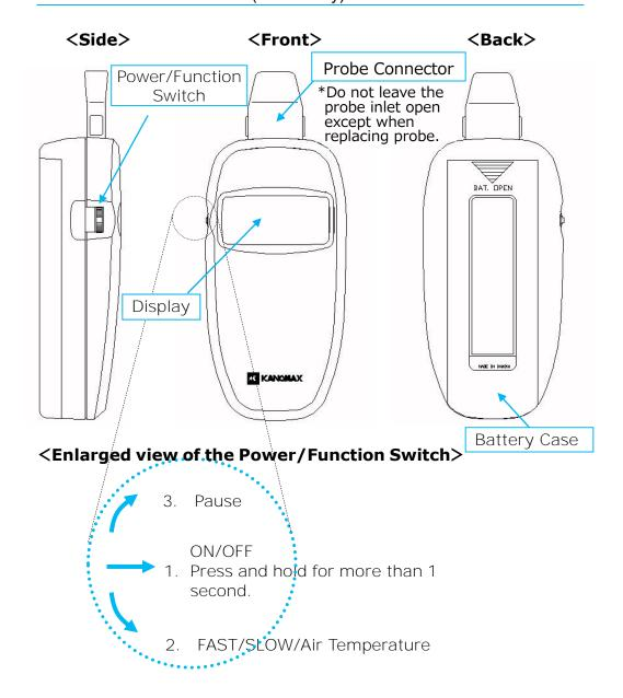
Power/Function Switch is a multifunction switch that can be slid up and down, and pressed.
