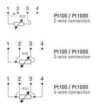
$^{\ast}$  Short terminals 1 and 2 on the transmitter, max 50  $\Omega$  on each wire
