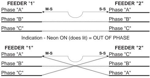
Note that the links must be arranged so that the phases are Connected in Phase, as indicated by the dotted lines.
