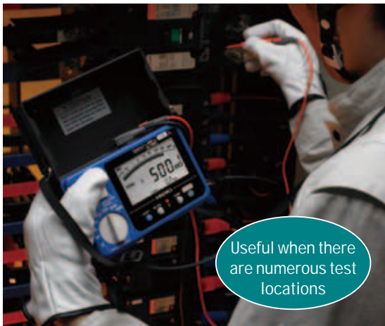
In some cases, the capacitance component may prevent a judgment from being made until charging completes.
