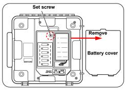
**3.** Disconnect the plug of the battery pack from the connector of the instrument.
