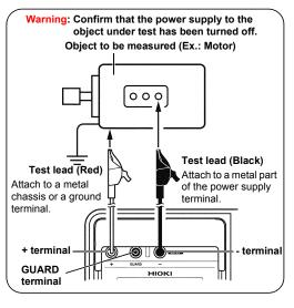
Clip the alligator clip at the end of each test lead to the object under test. 5. key, after which the Press the TEST VOLTAGE voltage display starts blinking.
