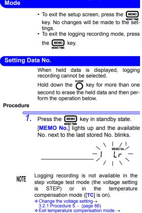
Exiting Setup Screen or Logging Recording
