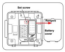
**3.** Place six LR6 alkaline batteries into the battery compartment. (Replace all six at the same time)
