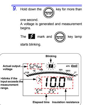
If > blinks, the input value is out of measurement range. Example: > 10.0 T $\Omega$  means "larger than 10.0 T $\Omega$ ."
