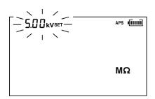
6. The test voltage is chosen from 250 V, 500 V, 1.00 kV, 2.50 kV, and 5.00 kV using the  $\bigcirc$  keys.
