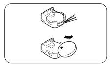
Insert tweezers or other similar pointed tool between the battery and the battery holder. Raise the battery to remove.
