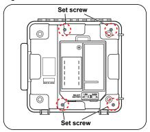
3. Remove the screw and pin holding the two printed circuit boards, and remove them.
