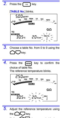
If the **O** keys are held down simultaneously, the reference temperature is returned to its default.
