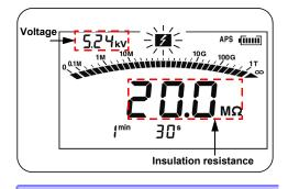
Stop insulation resistance measurement.
