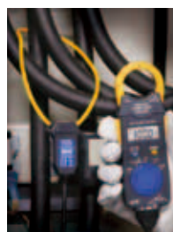
Use with an AC Clamp Meter to measure large wires and currents.
