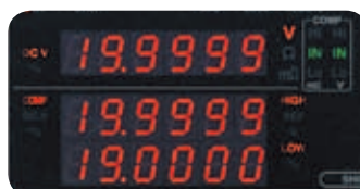
Voltage comparator settings
